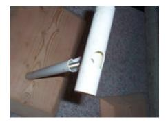
The sconce will use two pieces of PVC pipe. One for the candle and the other for the corpse arm. The Candle is made from a piece of 1 1/4th Schedule 40. It is cut to a 6 inch length and then a hole is drilled completely through both sides. One side this hole will be for the rod. On the other side it is used as a guide for a 1 inch hole. This hole will be for access so that you can install the light fixture and connect the wiring.
