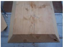
The plaque is made from a piece of two by 12 inch board. It was cut to a 16 inch length. I chose a 2 inch thickness to give the plaque a heavy look. Something that you might find in an old castle dungeon. The sides where all then cut to a 45 degree angle to give the plaque a finished look. Once that was done I needed to add the hole for the rod that the wire will run through. I measured to find the center of the board and then up 3 inches from the top of the bottom edge bevel.
