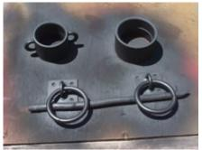
With the shackle made you can paint the hardware. Flat black spray paint is used . Once it is dry slip the shackle over the arm and drill a small hole in it. This will be to hold the shackle with a screw. In the picture the hole is on the top. It should be screwed in under the arm. This gives the appearance that the shackle is being pulled up by the chain.
