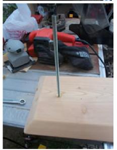
Now the rod can be installed. It was a tight fit, so tight that I needed to screw the rod in. Once it was through I installed the locking nut on the front and a washer and nut to the back. At this point you may want to stain the plaque.
