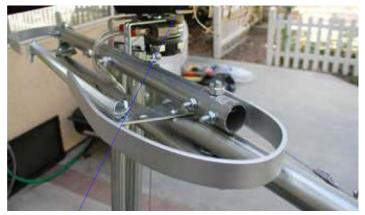
In this picture is a close up of the left shoulder mechanism.
