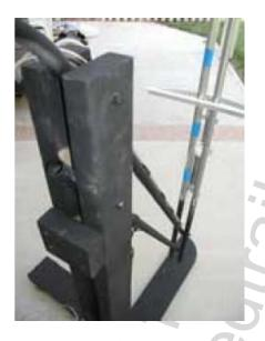
The 4-bar linkage consists of a pair of 2x4s in which a pair of 3/4" electrical conduit tubes pivot. I chose electrical conduit because it's fairly light weight, cheap, easy to work, readily available and strong
