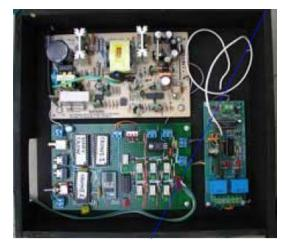
At left is the electronics package. It consists of a 5/24 volt power supply (upper), a receiver for the remote (right) and the main circuit board.
