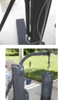
A rotary actuator is just a pneumatic cylinder that rotates. I got this one off Ebay for about \$15. It has an adjustable angle of rotation, but I use it for the maximum 180 degrees.
