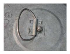
As purchased from the store, the handle for the trash can is merely crimped on the lid. To the left of center is a pop-rivet that helped hold things together during construction. To right of center is the threaded end of the bicycle tire pump, with a nut on the end.
