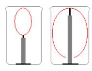
The pumpkin on the left has the piston mounted to the bottom. The pumpkin can be no larger than half the height of the trashcan because of the height of the pneumatic cylinder.
