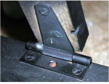
The wooden lever is attached with a plain "T" hinge.
