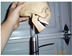
Using cable ties, I attached the air cylinders to some EMT pipe that was pounded into the ground behind some of the tombstones near the driveway, which effectively scared everyone approaching the house!
