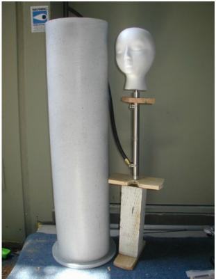
Pneumatic cylinder and blocking inserts in the column, so the top of the styrofoam head is flush with the lid.
