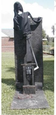
From behind, you can see how we mounted the rotisserie motor inside a wooden housing we constructed. We had to leave enough space from the ground so that the swing arm didn't hit bottom when it rotated underneath.
