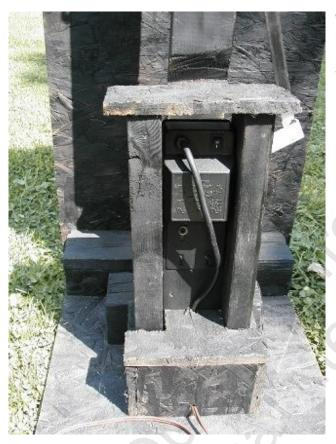
We used the bracket that came with the rotisserie motor. It was a universal mount for gas grills. Here is a closer view of the motor from behind.
