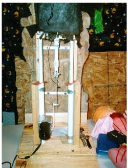
I added a piece of 1/2" in middle of the hole, Then a coupling, and a short piece of pipe cut out for linkage. The longer the pipe in center holt, the shorter the linkage. Don't get it too short it will bind up.
