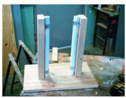
I centered the 2X4's,fitted the skeleton pipe so it slid up and down smooth and screwed them to the plywood.
