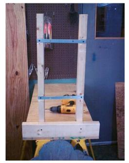
I built a frame to hold tombstone, I want mine attached, all one piece. Notice the metal bars have holes in them. I placed the cut out board on frame and drilled holes.
