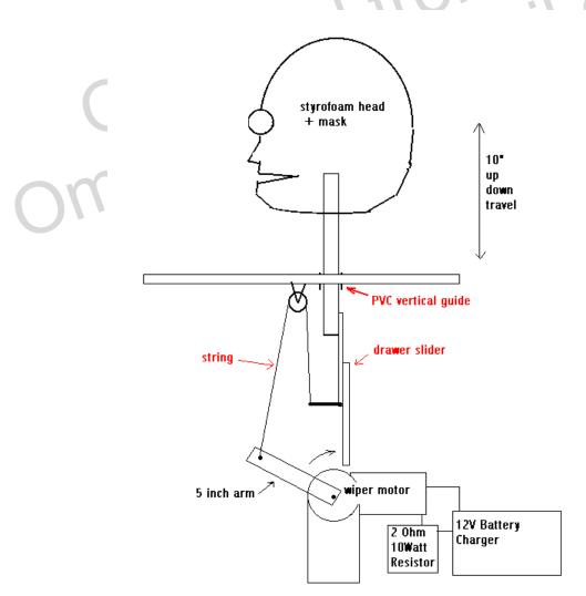
I think going towards a string and pulley mechanism would run much more smoothly and reduce the friction. I think a drawer slider would work well to restrict the motion vertically. I haven't built this but it would probably run better.
