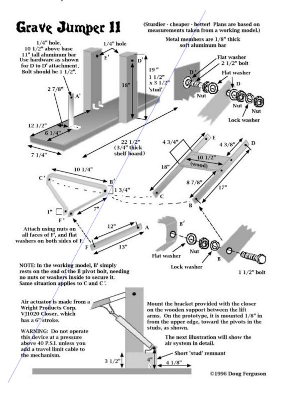
Obtained from Omarshauntedtrail.com The present device, besides being much less expensive to build, adds a slight twist: The head, instead of simply hopping straight up, leans forward slightly as it jumps. As the normal practice of halloween-l imagineers is to use door closers for pneumatic cylinders, we can't normally get the 'long throw' that a more expensive pneumatic jack can provide.
