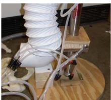
The 2.5 inch PVC elbow was used to channel the fog front the fog machine into the flexible vinyl dryer ducting.
