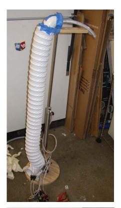
In the extended state, the vinyl dryer ducting takes the glycol fog into the head/mask without much condensation loss
