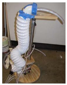
The basic mechanism inside is a 20" stroke air cylinder for vertical movement of the dragon head and two little 1" stroke air cylinders to tip the cylinder forward
