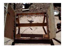
Attach the hinges to the frame and the doors then mount the motor I used a motor from a rotisserie I got at a yard sale
