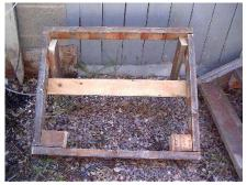
Take the single 34 1/2 in board you cut earlier and attach it to the back of the frame for the motor support
