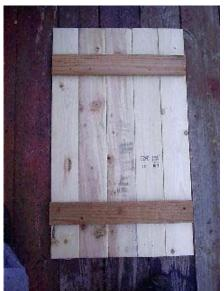
Then cut one 6 foot board into 2  $\,35$ in sections put five of the 2  $\,\frac{1}{2}$  ft sections together and nail or screw them to two the  $\,35$ in sections you cut
