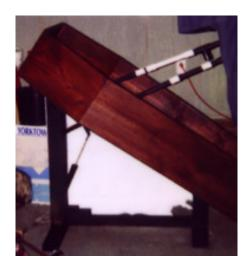
Here's a (somewhat) closer view of the mechanism. I'm using a heavy-duty screen door closer as the air cylinder.
