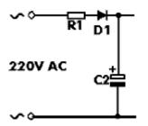
In Europe, the line voltage is sufficient to drive a xenon tube after rectification. This is a typical power supply for a line-powered strobe in 220 Volt countries.
