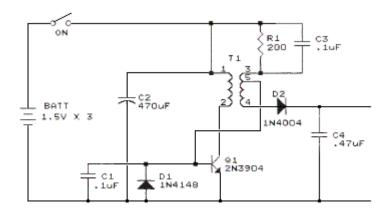
Battery-powered strobes are much more complex, due to the effort required to boost battery power up to a suitable operating voltage.
