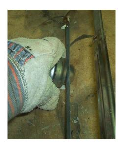
Cut off the top part of the wick assembly with a hack-saw. Use gloves for hand protection.
