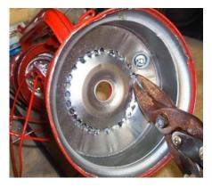
\* \* This part is optional. \* \* I thought I was going to use a large bulb for the light. So I thought I need to enlarge the opening. I drilled a bunch of holes then I cut them with some old tin snips.
