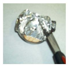
Drill a 1/4" hole in the wood. Then place the wood in the underside of the wick piece. Then tape it down using the foil tape. Here, I am trimming off the excess tape. (sorry about the blurry pic)
