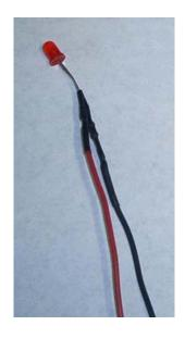
Cut the wires back on the resistor to about a 1/4". Solder the resistor wire (it doesn't matter which way it is facing) to the short wire of the LED. Then solder the other end of the resistor to the BLACK wire. Solder the RED wire to the longer wire on the LED. Place the Heat Shrink Tubing over the connections and lightly run your soldering iron over it to shrink.
