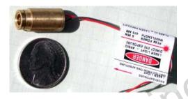
LASER diodes are also available built up into "modules" that contain the LASER LED, driving electronics, and lenses.
