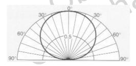
This radiation diagram shows the output of a green LED with a diffused colored case (Photron PL-GB574G).
