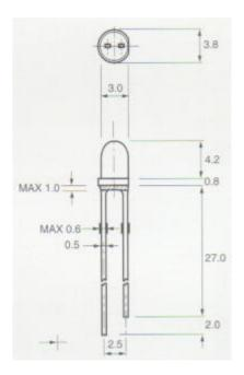
Dimensioned drawing, from the Photron catalog, of the standard LED size called T1. All dimensions are in mm.
