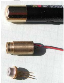
As of this writing, commonly available LASER diodes are confined to the red and infrared portion of the spectrum. Laboratory prototype blue LASER diodes exist, but have short lifetimes, or need to sit in liquid nitrogen. Green LASER diode assemblies exist, but they cheat: an infrared LASER diode is used to pump a frequency-doubling crystal.
