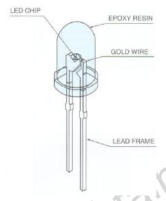
This drawing, from the Photron catalog, shows the anatomy of a common LED
