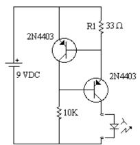
The current is set to V<sub>BE</sub>/R1, where V<sub>BE</sub> of a 2N4403 transistor is a minimum of .75 V and a maximim of .95 V. Depending on exactly which transistor you use, a little fiddling with R1 can be set to any convenient current. [David threw one of these together with junk box parts and it delivers 17 mA, which is close 2N4403 enough.]
