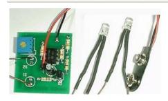
The circuit provides two LED eyes that can be adjusted between a slow fade-in/fade-out to quick pulses. The speed is changed by adjusting a variable resistor with a small screw driver.
