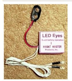
The circuit provides two LED eyes that brighten and dim automatically.
