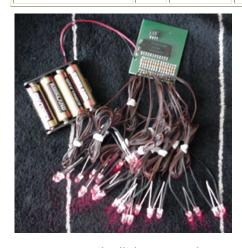
The circuit controls 15 pairs of L.E.D.s that look like beady little rodent eyes. All the eyes are normally on, with one pair at a time blinking off in semi-random fashion, as if the animal had to close its eyes briefly.
