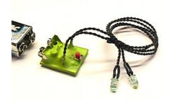
The circuit provides two LED eyes that can be set for various effects.
