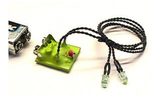
The circuit provides two LED eyes that automatically change color.
