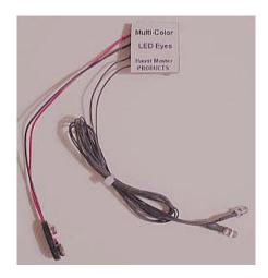
The circuit provides two LED eyes that change color automatically.
