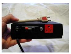
This is the rear of the control box, showing: fuse, speaker-level audio input, indicator lamp, and socket for the flash head.
