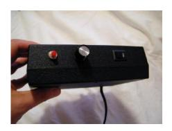
The front of the controller has: test switch, sensitivity control, and power switch. The power switch also contains a pilot light.
