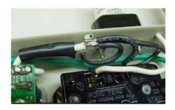
8. If you have some heat-shrink tubing, slide a piece over the white wire as shown. Solder the 3 black wires to the white wire. Slide the tubing over the wires and shrink it. If you don't have any tubing, use electrical tape to completely cover the junction. You don't want to energize the metal housing.
