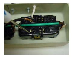
3. Open the back of the strip to expose the sockets. Using a small screwdriver press on the tabs to release the white wires. The picture shows a black wire, but you get the idea. The white wire in this pic is actually the wire from the starter socket.
