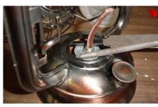
Using a screw driver, file or what ever will fit, to hold the washer in place until is dries.
