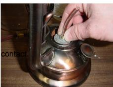
Push the cord and washer assembly back into the wick opening.
