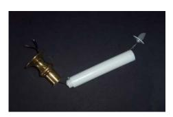
Next, pass the flex through the candlestick, the brass holder and the tea light top, and solder the flex to the base of the tea light. Test the bulb at this point to ensure that it is working!
