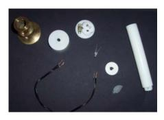
Then unsolder the wire from the LED and the tea light base. You now have the components for rewiring and assembling the flickering candle.
