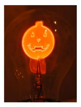
This display results from <u>flat plate electrodes</u> in the shape of a pumpkin, with cutouts for the eyes, nose, and mouth.
