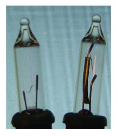
\*\*\*Here is the deal, You need *Twinkle* bulbs. They are easily confused with a flasher bulb. They do almost the same thing, Flash on and off, but a Twinkle bulb has a little jumper built in so that when the bulb goes off the strand doesn't lose power. Where as a flasher will cut the power to whole strand.
