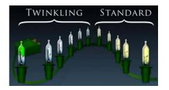
Pull all the Twinkle bulbs out of the twinkle strand, just pull them out of the socket, and replace the first six or seven bulbs of the Standard Strand with the Twinkle bulbs. Plug it into a dim able circuit and viola. Hide the flicker bulbs in a box, with vents, out of view.
