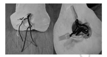
Tuck the wire connections into the bottom of the candle set and secure with a good amount of hot glue. Also put a ring of hot glue around the top of each socket to keep it from twisting in the candle when the bulbs are installed or removed.
