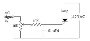
This is the low-frequency channel of the Ramsey Electronics #ML-1.
