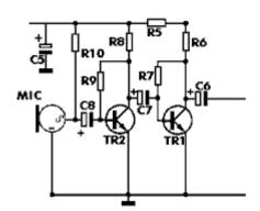
This is the input side of <u>Smart Kit Electronics</u> SmartKit #1014D. It uses an electret microphone and a two-transistor amplifier.
