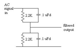
We really have a resistance and capacitive reactance in parallel. Ultimately, it provides a combined resistance with a value depending on the frequency of the signal.
