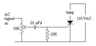
This is the high-frequency channel of the Ramsey Electronics #ML-1.
