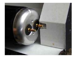
You must carefully align the ends of the lamp so that the two pins are in a line with the slot. Once the pins are properly aligned, slip the lamp into the fixture. Slide the right pins into the right slot, and the left pins into the left slot at the same time.
