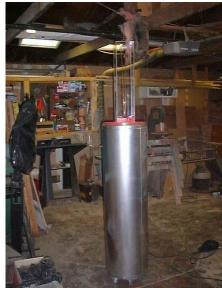
The first thing I did was to paint the outside of the water heater silver. I did 2 coats of paint on this but only used one can of paint as silver goes a long way. Then I cut a piece of 3/4" plywood for the top and cut a hole out of the middle for the flue pipe hole.
