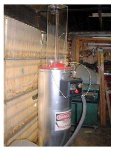
Then I attached a piece of 2 x 4 over this hole this is the mounting block for the Jacob's ladder wires. I used 8 gage wire for this about 30" long that are screwed into connector blocks on the 2 x 4 block. I painted this part red and made a Plexiglas box to fit over the Jacob's ladder. To weld the sides of this together I used my soldering iron and melted the pieces together with butt joints. Then this was screwed to the 2 x 4 block on top of the plywood.
