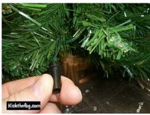
Everything is held together with either Hot Glue or Wire Ties. The Sensor is held on to a branch with hot glue. Wiggle and gently pry the sensor off he branch. (you can see on the right branch where the glue is).
