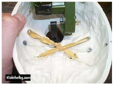
This is a view of the completed jaw tension setup. This is where you have to experiment a bit. I played around with the rubber bands by tying and untying knots in them to increase and decrease the tension. Adjust them so that the jaw stays closed BUT so that only light pressure is required to open the jaw. THIS IS CRITICAL as the servo doesn't have a lot of gusto.
