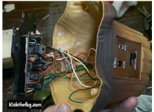
I drilled a hole next to the side panel so that I could get some cutters in there to remove the panel.
