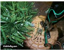
Remove the screws that hold the bottom panel of the tree. Carefully remove the panel with all the crap attached to it.
