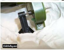
This is the desired end result. Pic1 is of the mounted servo with the arm on the servo sticking out the hole. Pic 2 (ignore the springs, pictures taken out of order) shows the bottom
