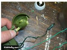
OK, lets trash the tree further. Pic 1 shows the eyes intact as they come with the tree. Remove the eye cover from one eye. (Pic 2). As you can see in the second picture, the green eye power wire runs through a hole with green Christmas bulbs at the end to light the eyes. We need to free up these wires so we can ditch the entire plastic eye assembly. We want to use the Christmas bulbs alone.
