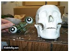
Now that you have your line secured in the bottom jaw with your screw, tie the other end to the servo arm (see pink stripe). Make sure there is no slack in the line. Line should be snug since when the servo arm moves it will pull your jaw open. When the servo arm relaxes, the rubber band tension we set up earlier in steps 41-43 will close the jaw. You see what I mean now about having the perfect tension?
