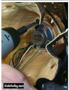
With the panel removed, remove the screws that hold the speaker.
