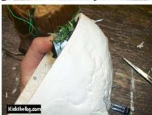
We are going to mount your servo in the skull next. As you can see I removed the glue and BOTH arms and mounted my servo. I later remounted and reglued ONE arm to the servo.
