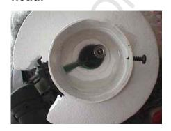
Here you see the view from the bottom of the wig head. You see the connector that will plug into the Santa neck connector and a small screw I added to tighten after the PVC is slid over the Santa neck stump.
