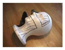
I've marked the section of the foam head I'm going to remove with a hot wire foam cutter. You can use a knife or hacksaw blade if you do not have a foam cutter.
