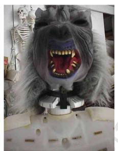
This photo shows the Dougie head with a mask and the PVC glued to the neck and attached to the Santa neck stump.
