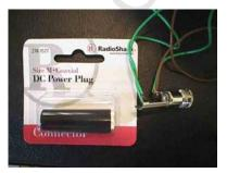
This Size "M" connector (Radio Shack part # 274-1577) can be attached to the wires from the hacked Dougie which will allow for easy plug in to the neck on the Santa.
