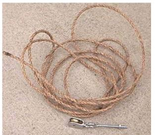
Here is the pulley and the rope. The pulley is attached to a 4" eyebolt that will be fasted to the top 2X4 of the guillotine
