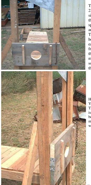
This is the stock end. It's made of 2 2X8s. There is a hinge on the left side of the stock. The chain on the right is nailed on with 1 big spike. The chain loops up on to another big spike on the right side. The chain has some slack in it so it hooks up on the top of stock pretty easy. The 2 upright pieces on the front of the stock are just nailed to the top of the stock. They're there mainly for appearance. I might put some metal loops on there later for them to slide down into.
