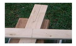
I started off by marking the center of the furring strips with a pencil so I could join them together square and true. I found the center of the shorter furring strip by dividing its length in half. The center of the longer strip is half the width of the furring strip itself. When you line up the pencil marks and square the two pieces at the top of the "T", you have have a nice, regular "T" shape.
