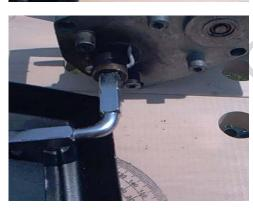
This is another pic of the nail through the driveshaft of the motor.
