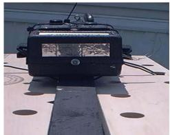
I then lined up the motor on top of the platform. Then I temporarily fastened the motor to the platform with black wire ties. Note the little silver screw about 1/2 way up on the end of the motor. I used it to fasten a steel bracket to keep the motor from shifting around while the crank was rotating.
