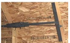
This is the steel bracket I mounted on the end of the motor to keep it from slipping around. The bracket was found at the lumberyard among the truss plates. Don't know exactly what this thing is called but it works great for this. I had to drill a hole to match up with the screw on the motor and for the three drywall screws I fastened it to the platform with. I put one of these brackets on each end of the motor. They keep the motor very still and no twisting occurs while its running.
