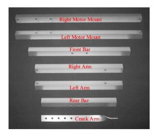
The 4' length of 1"  $\times$   $^{1}/_{8}$ " angle aluminum is cut into,
