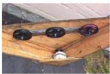
Problem was it becomes kind of expensive, inefficient, and messy with all the added motors, lines, and pulleys. To solve this I came up with a portable drive-unit that runs 3 separate paths/lines from one motor source.
