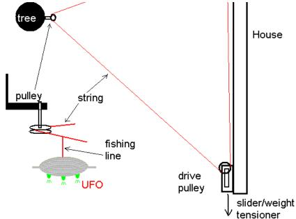
Yard picture of triangular track. Slider provides constant tension to the string and allows for elasticity of line and continual stretching of string due to tension and humidity. In previous years we had problems keeping string on the track because it lost tension over time. The dummy pulleys have to hang from a bolt, so that as the UFO goes around the pulley it does not catch on anything.
