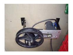
The original mounting brackets were intended to mount between rafter trusses but a better location required a change in mounts. Here it is in place. The driven line goes around this wheel to another idler wheel of the same size on the other end.
