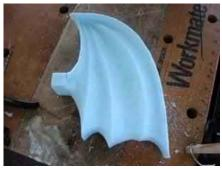
Shape it with the file, glue the middle body to the butt, shape them with the dremel, and finish up with the sandpaper.
