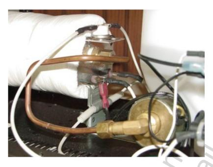
Next take the other lug and connect it to the other terminal where the pump was connected. This is blue lug. This is right on the plug where your remote would go.
