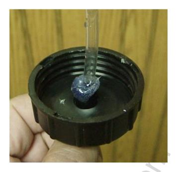
Hook up the pump and put the check valve in place.
