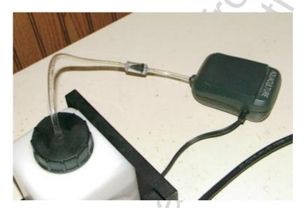
As usual before you piece it together test it first. Hook up your remote and power it up. The pump may hum a bit before you actually push the button because there is a bit of voltage on the line while it's warming up. Once you get the ready light push the switch. This should work just like before and you will not be able to trigger the fogger until the ready light is on. After you find it's working fine put everything back together.
