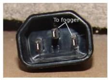
I picked up an <u>IEC extension cable</u>, which has the kind of connector my fogger control button has. I cut the other end of the cable off so that I could get at the wires.
