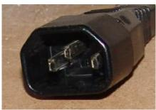
Next, I opened up button controller that came with the fogger. Using my multimeter in "continuity check" mode, I determined which 2 pins of the connector were connected to either side of the button in the controller. I have no idea how standard this configuration is, but in my case, it was the middle pin and the right pin, as indicated in the picture:
