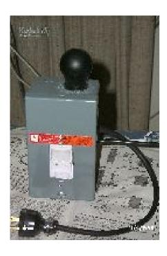
I purchased two F-70 fog machines this year. They have a wired remote control with a single button that you press when you want fog. But I did not want to stand around waiting to press the button till the TOTs arrived, so I built this automatic button presser.
