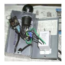
The wiring is simple enough for anyone to do. The IR motion detector has three wires, a ground, and two black wires (the black wires are interchangeable). My fogger uses 1/4" phono plugs, but I understand that other foggers use different connectors, so you are on your own there.
