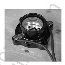
Inside the head at the top mount the socket base with hot melt glue. Hot glue is use to speed up the construction process. Also cover over the screw/wire connections with hot glue.
