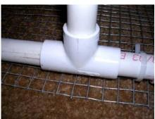
Using the 90 deg and T fittings, join all the pieces together and check for fit in the cooler. Once you are happy with the fit, bond everything using PVC glue.
