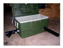
The Fog on the Rocks chiller is a great design by Deathlord. Its cheap to build and works really well. Throw in a couple bags of cheap cube ice and you can chill fog for hours. The particular chiller design works best with fog machines under 700 watts. If you have a larger fog machine, you should check back in a few weeks for a larger garbage can based chiller I am building right now. I plan on putting a full how to on the web for it soon. Anyway.. lets get building.
