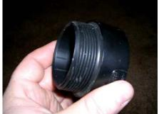
You will need a 2 short lengths of Black ABS pipe cut - figure 2 1/2" each. Take your PVC primer and glue and glue a male 2" threaded/slip fitting on the end of each 2 1/2" piece of pipe.
