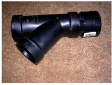
pipe. Glue the Y pipe with your PVC glue to one side of the 2 1/2" piece of pipe, and glue the fitting to the other side. This forms the inlet pipe.
