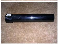
The output pipe consists of two pieces: A female 2" threaded/slip Black ABS fitting, and a 1 ft section of 2" Black ABS pipe. Glue the Female fitting on the 1 ft section of pipe using your PVC glue as in the picture below.
