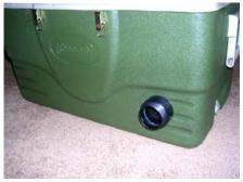
The center of the hole on the long side of the cooler should be 3 3/4" from the bottom of the cooler and 3 1/4" from the side. The center of the hole on the short side of the cooler should be 3 3/4" from the bottom of the cooler and roughly centered between the two sides.
