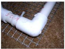
Next break out the hardware cloth (chicken wire like mesh) and cut a piece the same size as the PVC tray. Zip tie the mesh onto the tray. Insert the completed ice try into the cooler and check for fit.
