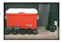
The first step is to cut a hole through each end of the ice-chest. We used a 4" bi-metal hole saw attached to an electric drill to easily cut perfectly round holes through the center of each end. These unique saw blades (Vermont American Tool Company) can be found at most hardware stores. The bits are a little expensive at around \$25.00, so an alternative would be to use a compass to the mark the circle for the hole and then use a jigsaw to cut it out.
