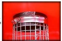
Using needle-nose pliers, bend those end wires you purposely left on under and over the lower screen wire to hold it in its tube shape (pictured center). If a few of these break off its not a problem, but if a lot break off you may need to use some lightweight bailing wire to re-enforce the seam of the wire cage. What you should have is a tube-shaped wire cage that is attached at both ends of the chest (pictured right). This is the chamber that the fog will pass through and be cooled in.
