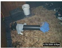
Here you can see my entire setup. You notice the previous mentioned rag on the fog machine end. I also added a rag to "slow" the escape of the fog from within the chiller. My fog machine is so forceful that some of the fog was coming out un-chilled. This method (though stupid looking) works very well.
