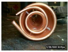
Now slide the smaller coil into the bigger coil. (see below)
