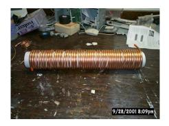
For the outer coil, I did the same using 50 feet of 3/8 inch copper and a 3 inch scrap piece of PVC. (Your hands will hurt after coiling this bigger copper!)
