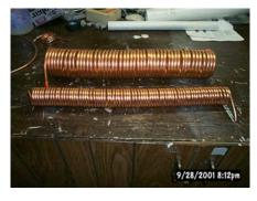
Once the coils were made, I pulled the scrap PVC out of them and spread the apart a bit like a spring till they were the same length as the stove pipe.
