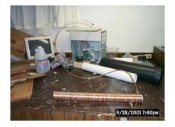
To build the inner coil, I took 25 feet of 1/4 inch soft copper tubing and bent it around a inch and a half scrap piece of PVC pipe. The soft copper bends well enough that it is easy to coil it around the pipe. As you can see I had a little left over.
