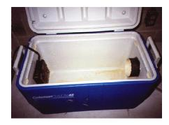
Install the 4" fan to the inside of the cooler that has the pipe flush with the inside wall. I used long skinny sheet metal screws to attach the fan. Be sure you have the fan facing the correct way so it is blowing out the pipe. On the other side of the cooler is where the for machine will go so the fan sucks the fog through the chiller.
