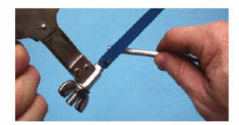
2c. Insert the rod and drill a small ½6" pilot hole through the rail and into and through the aluminum rod. Drive a nail into the hole and through the rod. This prevents the rod from swiveling in its hole as you cut in different directions.
