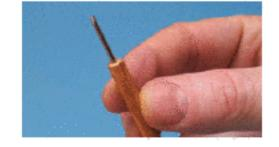
Place the dowel in any pegboard hole. The distance from the wire to the pin will be the radius of your circular cut. Energize the wire. Slide a piece of foam into the wire and impale the foam on the pin. As you spin the foam around on the pin, you'll cut a perfect circle. Turn off the wire and remove your part.
