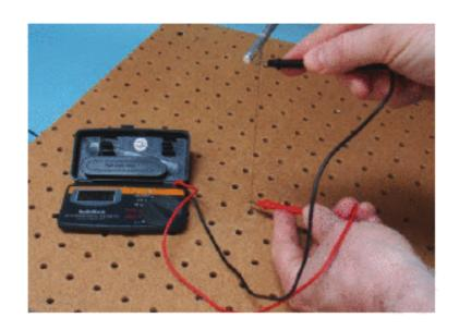
So the current needed is just under 2 amps. My train transformer is rated at 2 amps, so that's good, at least for short time periods. The resistance of the wire will change at various temperatures, so the current drawn will vary. Many train transformers have a built-in thermal breaker — if they get too warm, they'll shut off. If that happens, unplug the transformer and let it cool down. It should work again later.
