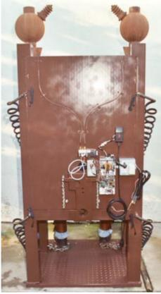
The lower (center) junction box hoses the First Step BASIC stamp microcontroller and the Radio Shack digital voice recorder.
