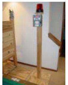
Here is the fake control box. I took a standard electrical throw switch and added a pneumatic cylinder to it to "throw" the switch.
