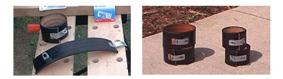
I found some small padlock hasps at the hardware store that were perfect to fasten the shackles. I drilled holes in the belt and fastened the hasps on with some tinner's rivets. The pic to the right is the finished hasps ready to be bolted on the electric chair.
