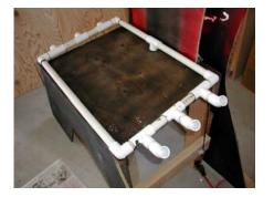
Here is the detail of the 3/4" PVC piping I used as the foundation for the legs. A series of "T" and "Elbow" connectors glued together and sized to fit under the seat. Note the one "T" in the back where the fog pipe will connect.
