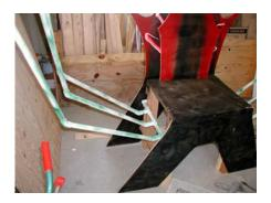
This pic shows the legs in place. By mounting the foundation piece under the seat, all the stuff is hidden. The legs are 2 foot sections on the bottom, and 3 foot in the middle and 3 foot on top. I used 45 degree elbows to connect them. The middle leg has holes drilled every 6 inches to allow fog to escape.
