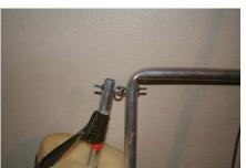
Connect the handle eye-bolts to the arm eye-bolts and crimp closed.
