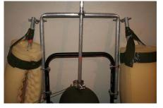
Using the two 5/8" pieces with the BMX handles, drill holes about 2" from the bend; this will give you a little extra leverage for raising the hands. Mount the eye-bolts with the holes pointing towards the body.
