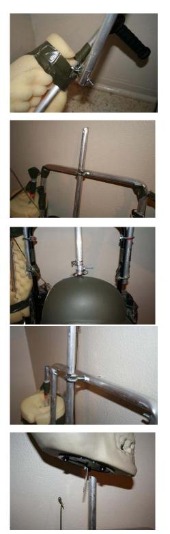
Mount the large eye-bolt at the center of the top rail between the shoulders. The hole must face forwards. This will support the neck tube and head.
